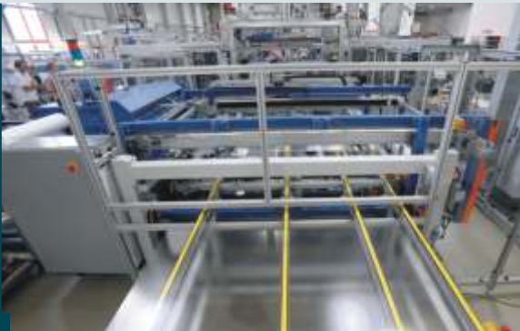
EVA foil sheeter combined with alignment unit
