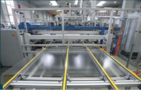
Feed conveyor for cleaned glass
